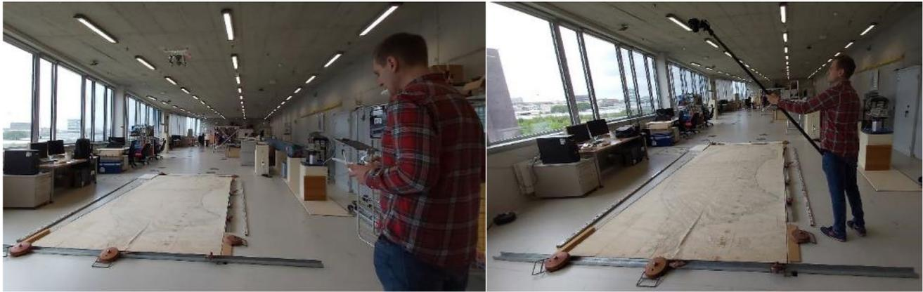
**Fig. 2** Image data acquisition with UAV system DJI Phantom 4 Pro (left) and with Nikon D7500 at the telescopic rod
