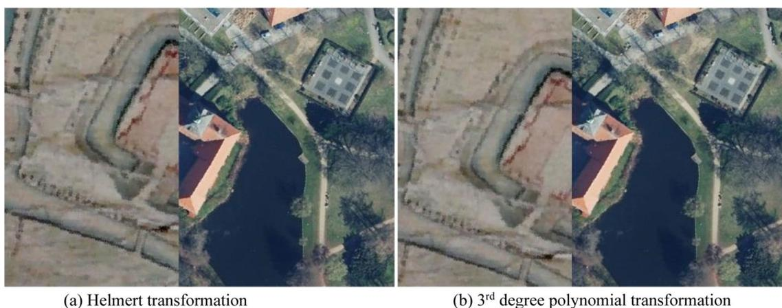
**Fig. 11** Visual comparison of the georeferencing result between Helmert transformation (a) and 3rd degree polynomial transformation (b) on the data set of the Nikon D7500 with a 50 mm lens showing a large offset in the map (left)
