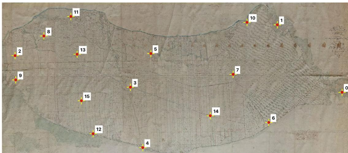
**Fig. 9** Overview of the distribution of all measured ground control points (note: map is oriented to the north here in contrast to Fig. 1)
