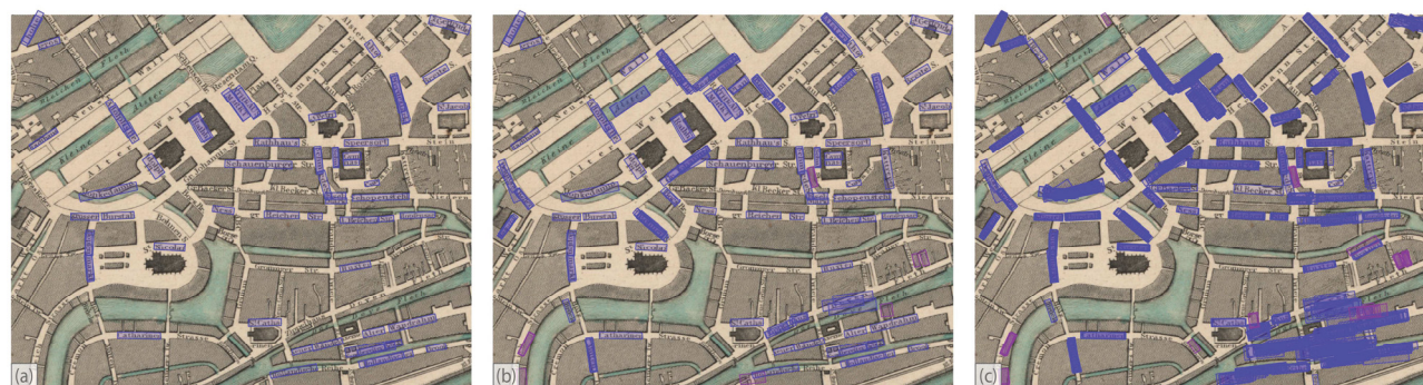
Figure 3: Detected text elements: true positives (blue) and false positives (purple). Strabo was applied to the original image subset (a), the combination of the original and the rotated input image through +45, +90, -45, and -90 degrees (b), and the combination of the original, rotated through +45, +90, -45, and -90 degrees, and enhanced (linear contrast stretching and global histogram equalization) input image (c).
