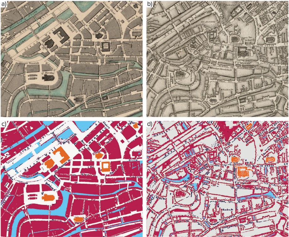
Figure 8: a) The original input map described in chapter 4.1 as well as b) a more complex, large-scale historical map (Harvard Map Collection et al., n.d.-b) showing the same spatial extent of the city of Hamburg. The OBIA workflow originally developed for map a) (see result in c)) was applied to b) and delivered less satisfactory results, as can be seen in d)
