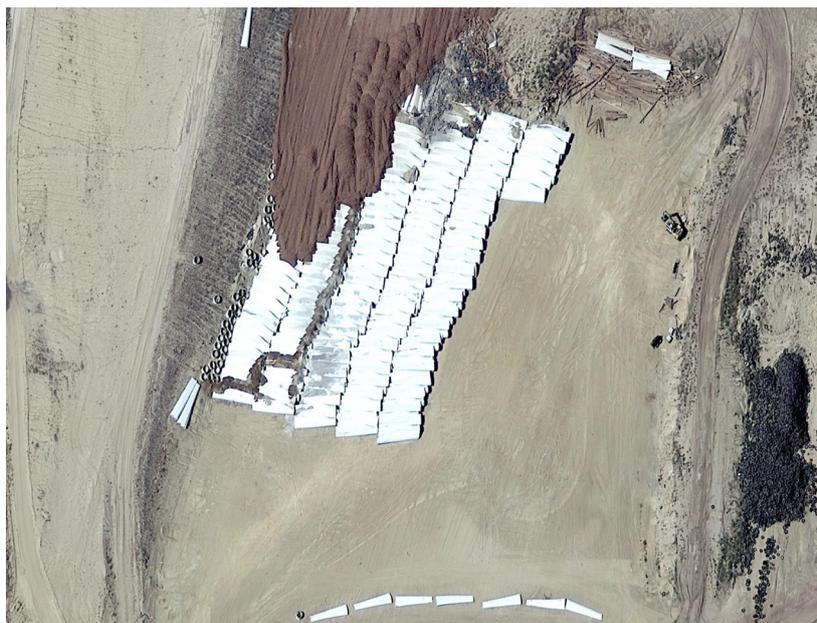
Figure 2. Satellite view of the landfilling of wind blades at Casper Regional Landfill in Wyoming, USA. The separation of materials in composites, used in wind blades, challenges their recycling (Image Source Google Earth. Image Date 02.09.2019).
