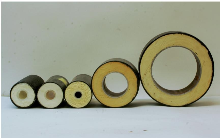
*Figure 4. From left to right: DH DN40 flexible plastic medium pipe and corrugated casing, DN40 flexible plastic medium pipe with smooth casing, and bonded steel medium pipes DN20, DN100 and DN200.*
