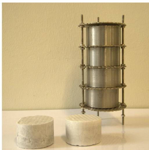
Figure 33. Sample holder with four moulds. Foam samples.
