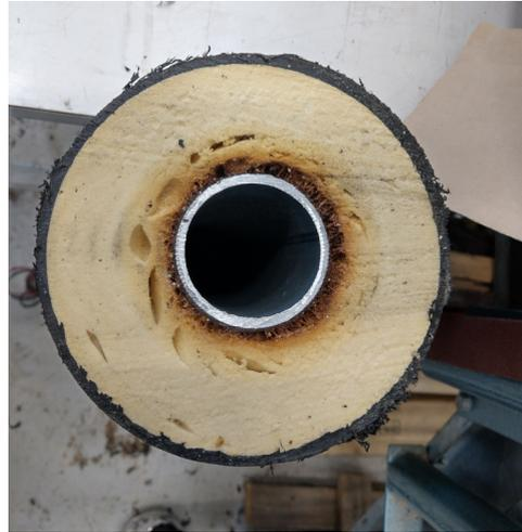
*Figure 6. Section of an aged DH pipe, showing browning of the PU in the vicinity of the medium pipe.
