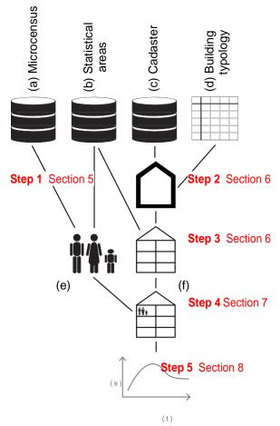
The diagram shows the three main databases (a-c) and the additional building typology used for the classification of the building stock (d). In step 4 the synthetic families (e) are merged with the constructed dwelling units (f). The simulation of heat consumption is performed in step number 5.
