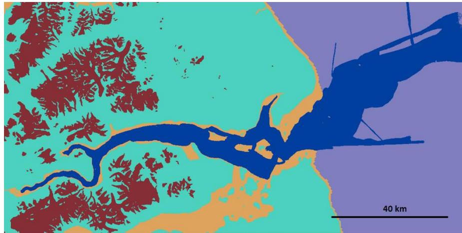
Figure 7. Splat map defining five territories: MSM66 bathymetry data (blue), IBCAO data (purple), transition (orange), the terrestrial elevation model (turquoise), and glaciers (ruby).
