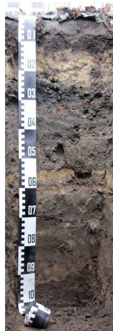
Fig. 5.10 Bore-hole: Anthropogenic soils
