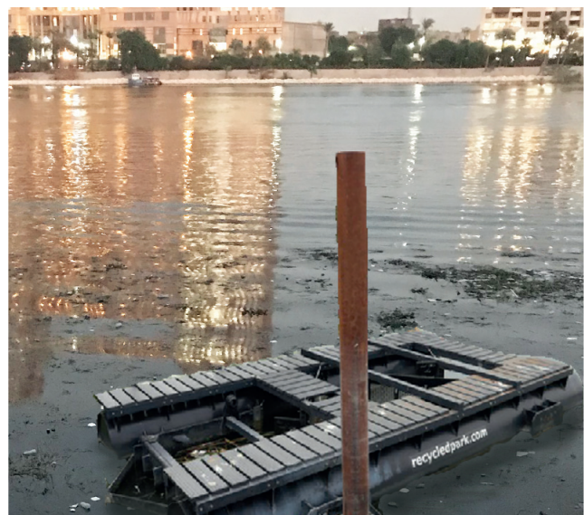
Figure 30: Collage of the litter trap installed where the plastic waste accumulates on the river. Source: Authors, 2019; with elements of the Recycled Island Foundation, 2018a.
