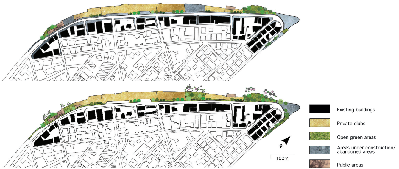
Figure 32: Land-use maps of before and after the project implementation with the indication of the places with the new landscape. Source: Authors, 2019.
