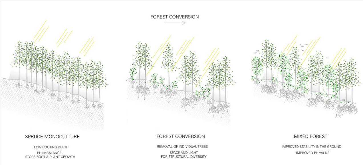
Fig. 31: The Processes of Restructuring the Forest Communities in Altonaer Volkspark (Gesche Delfs and Sarah Schmidt, University design Studio, HCU). The fast ecological processes in urban forests are steered and curated by maintenance and management regimes. In Altonaer Volkspark, these processes started with the vision to develop a Schönheitswald - a beauty forest. This entailed transforming a dense monocultural conifer forest into a mixed light-permeable deciduous forest.
