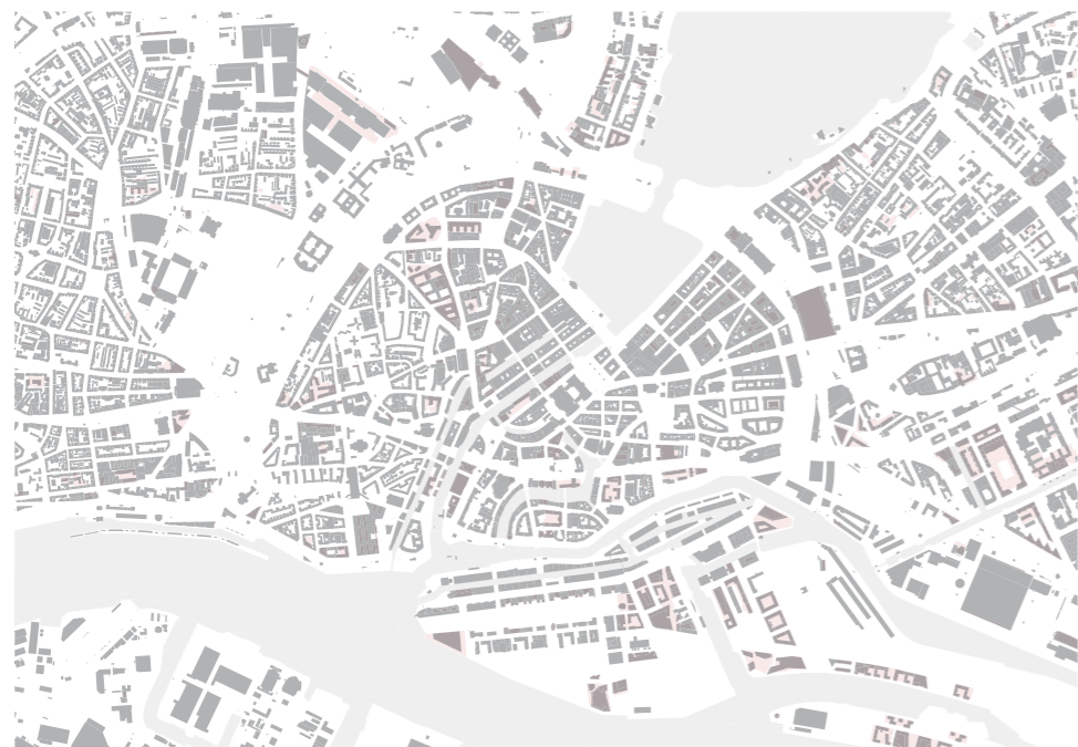
Figure 16. Visualization of polygons with the attribute AX_Gebaeude (buildings) in dark grey at a scale of 1:30.000. The map shows the building footprints in Hamburg Altstadt (author, 2025).
