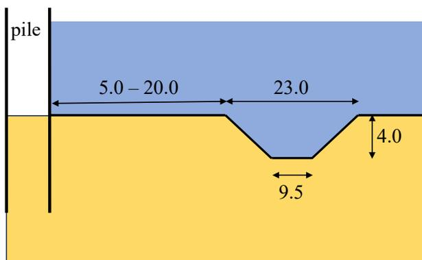
Figure 3. Geometry of the footprint and distance to monopile.
