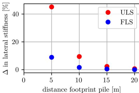
Figure 6. Change in lateral stiffness at the seabed level for multiple distances between monopile and footprint.
