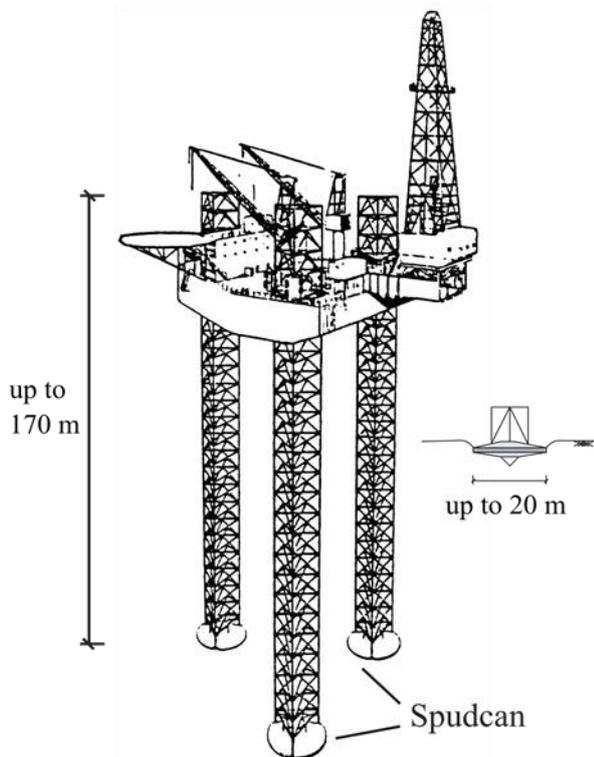
Figure 1. Illustration of a jack-up platform with three legs and spudcans including a detailed spudcan with central tip (modified after Reardon, 1986).
