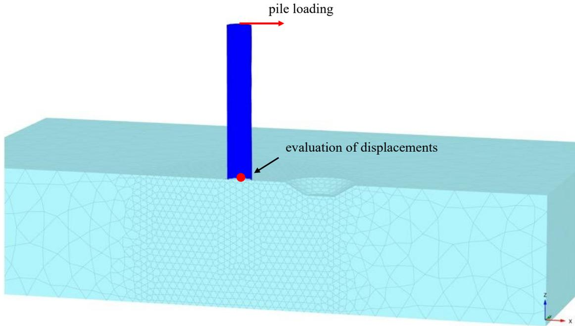
Figure 2. Numerical model of soil and pile including a footprint in 15 m distance.
