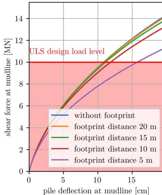
Figure 4. Load deflection curve for ULS load level considering multiple distances between monopile and footpad.
