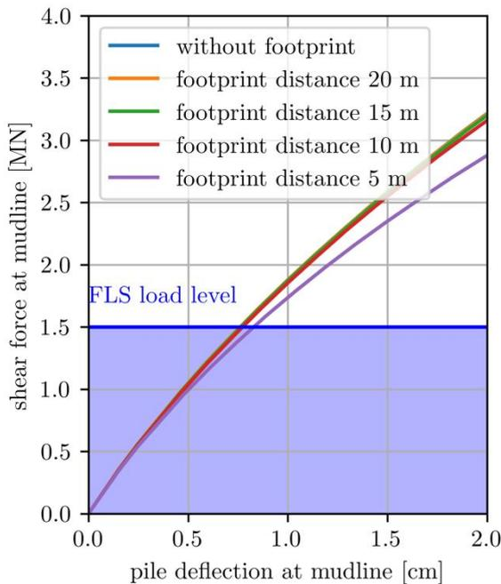
Figure 5. Load deflection curve for FLS load level considering multiple distances between monopile and footprint.
