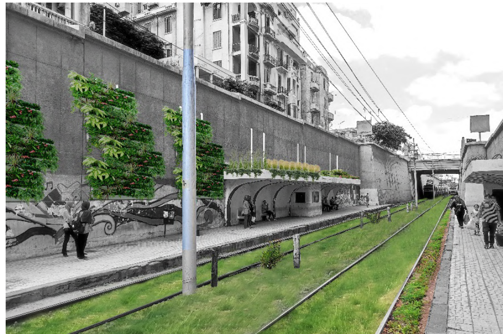
Fig. 5-35: Proposed integrated concept of bioretention street planter, green wall and green track systems for lower tram profile Illustration by Mohamed Elfouly on photo by Author – Cross section by Author
