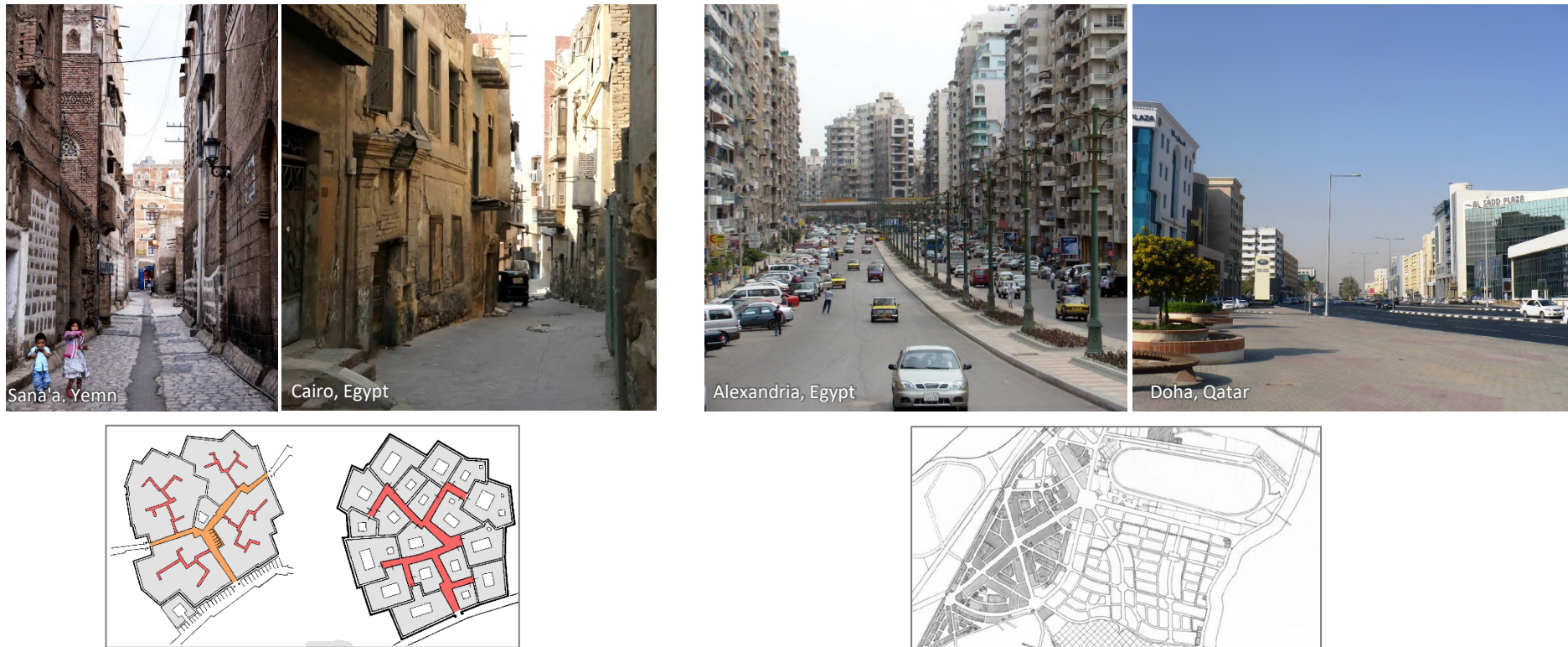
Fig. 2-12: Comparison between traditional Street network and hierarchy (left) and modern street layout (right).
