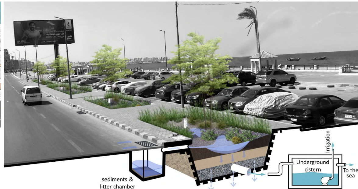
Fig. 5-41: Proposed integrated concept of bioretention planters and storage tanks systems in surface cluster example area (Illustration by Mohamed Elfouly on photo by author)
