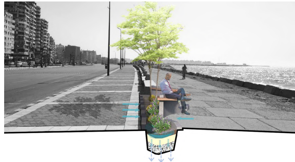
Fig. 5-42: Proposed concept of bioretention planters in surface cluster example area
