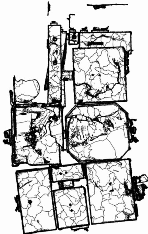
Fig. 2.6.29: Screenshot Archicad, 1F of first scan set with wrong angles
