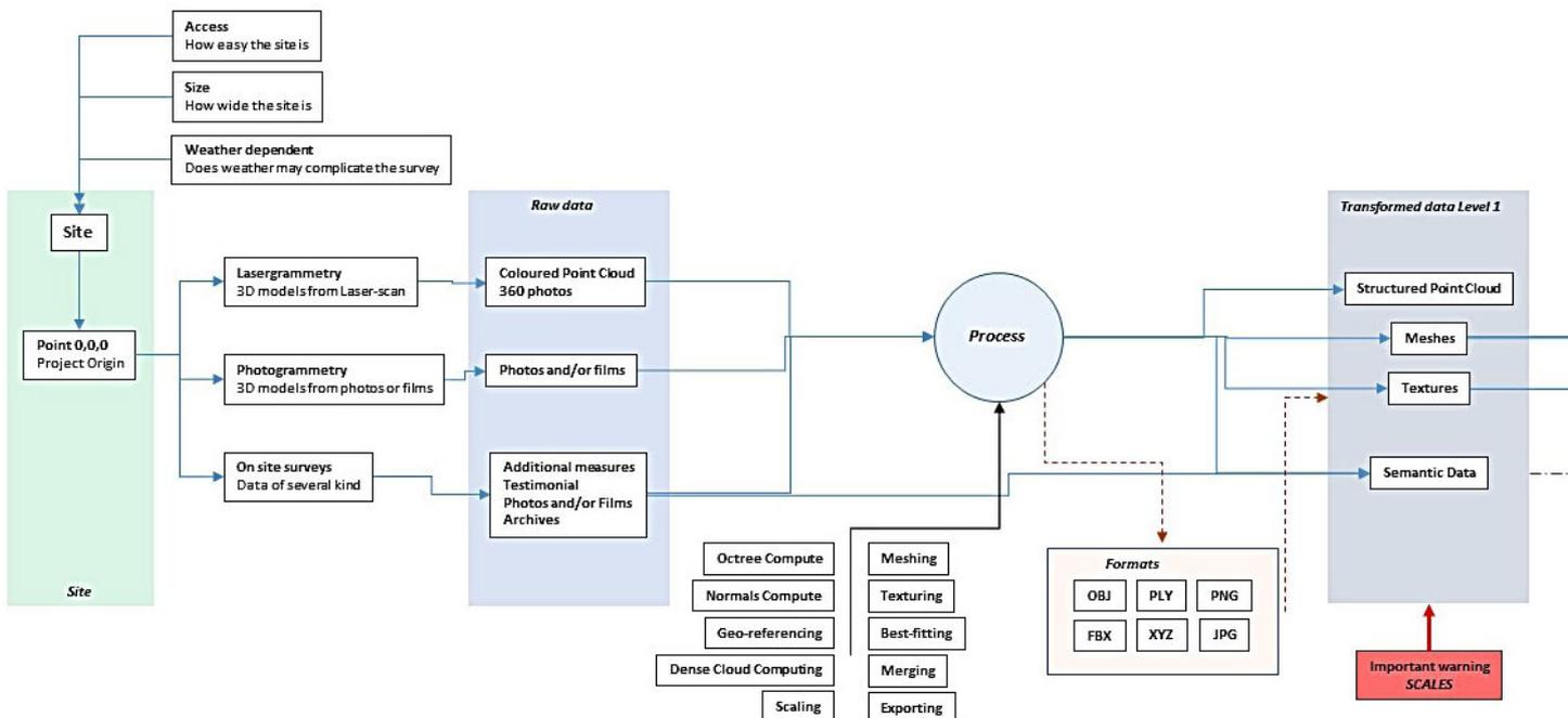
Fig. 1.1.3: Synoptic view of the data workflow
