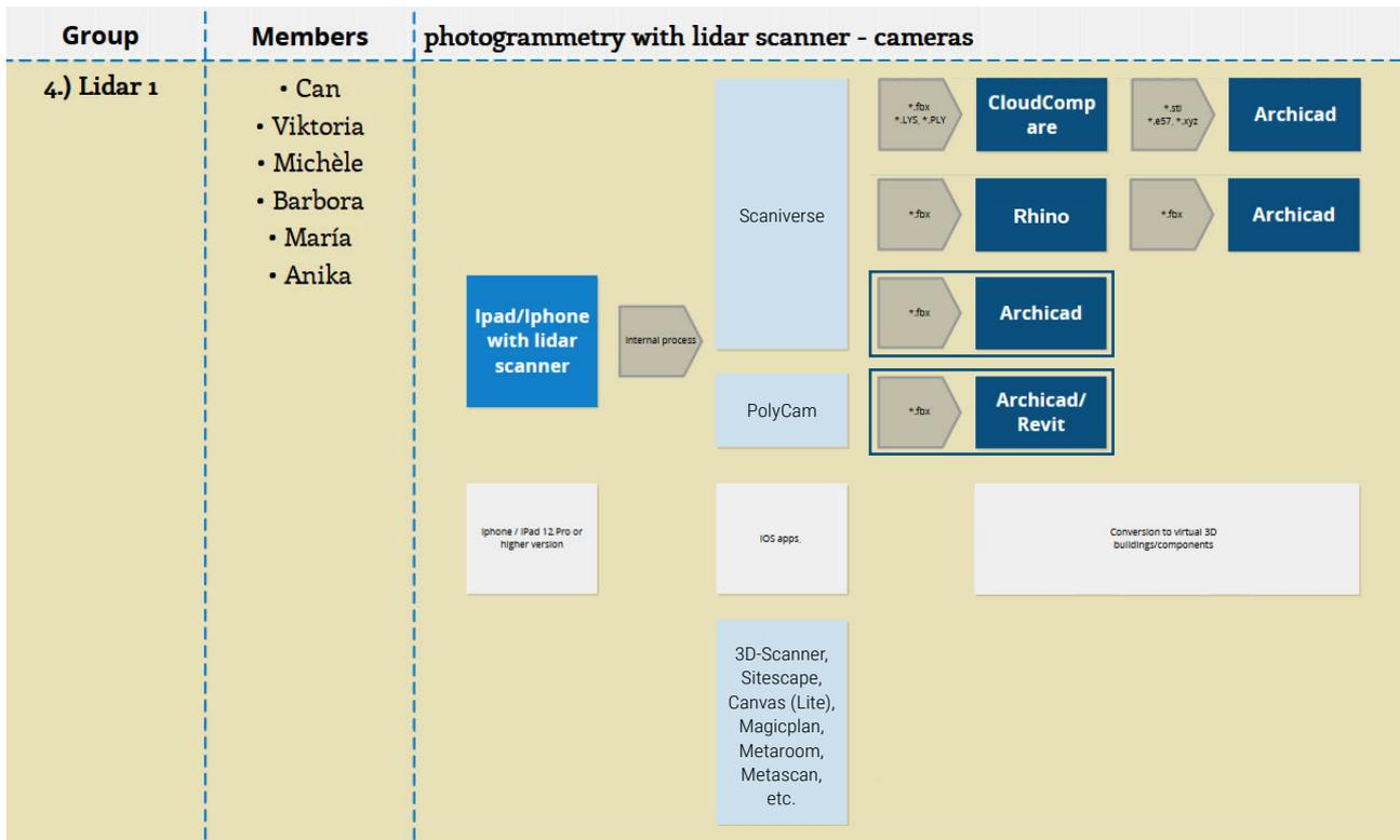
Fig. 2.6.3: Workflow LIDAR
