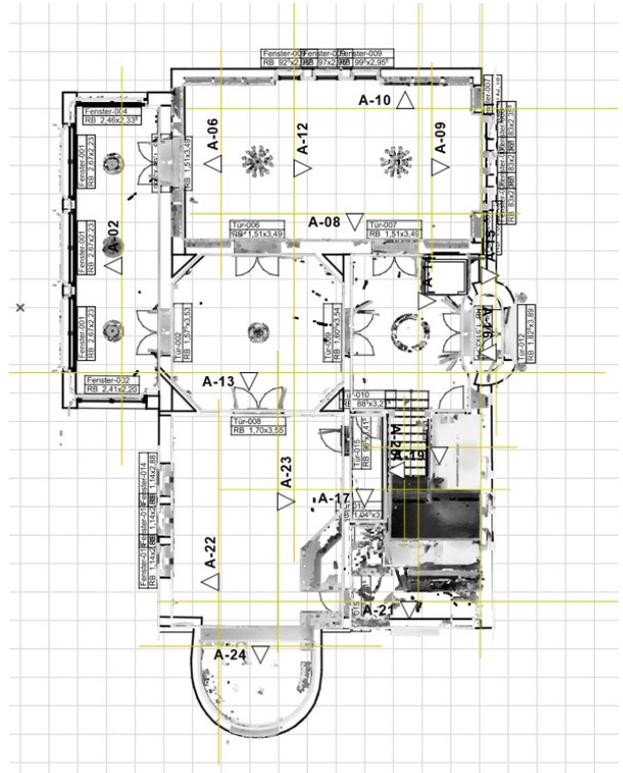
Fig. 2.1.22: Reconstructed floor plan with point cloud in the background
