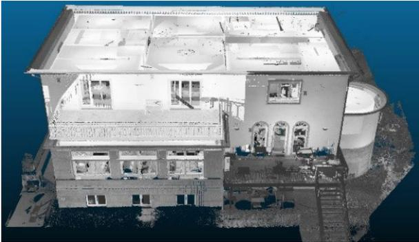
Fig. 1.2.9: Segmented point cloud from terrestrial laser scanning
