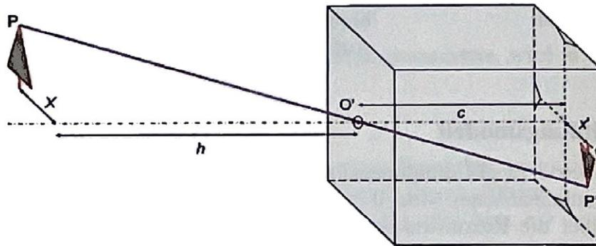
Fig. 2.4.2: Model of the pinhole camera <sup>2</sup>
