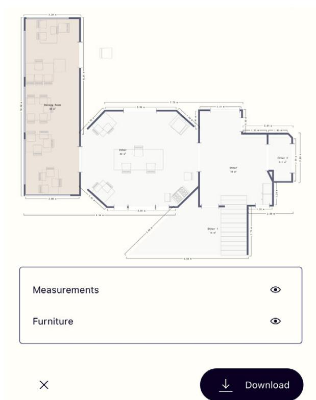
Fig. 2.6.59: Screenshot PolyCam, output of dimensioned floor plans
