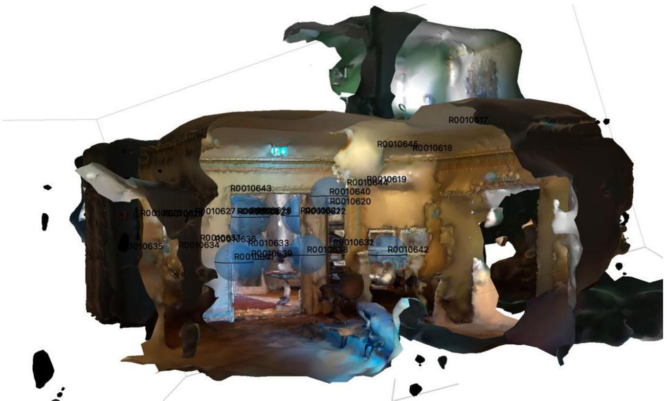
Fig 2.5.5: Representation of the vestibule, ground floor in Metashape with 30 photos; Attempt 2
