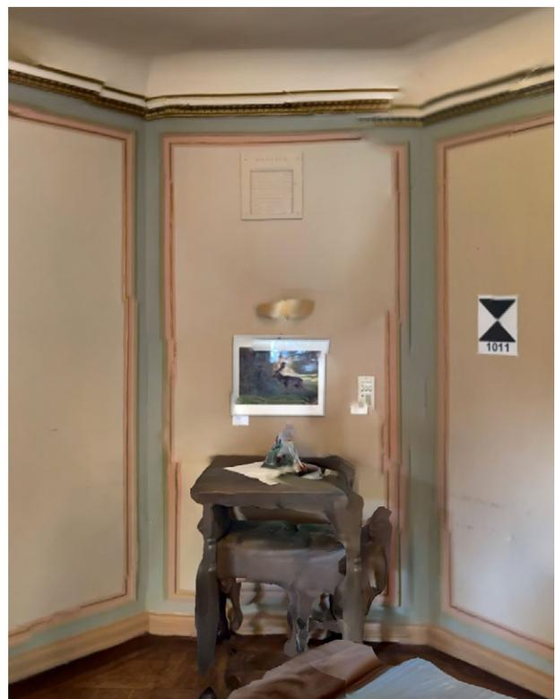
Fig. 2.6.22: Screenshot Scaniverse, misalignment of stucco mouldings
