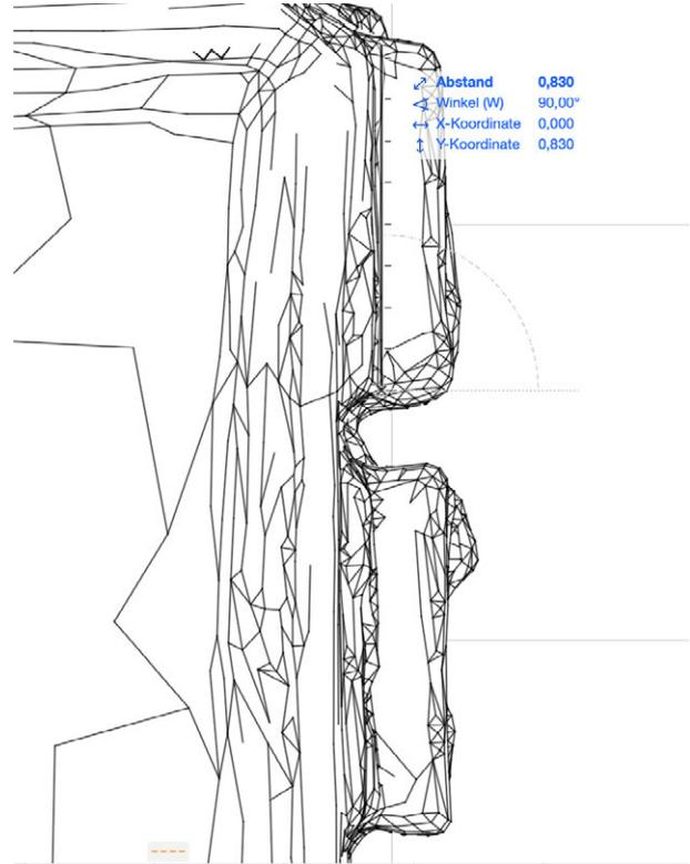
Fig. 2.6.41: Screenshot Archicad, measuring the window width
