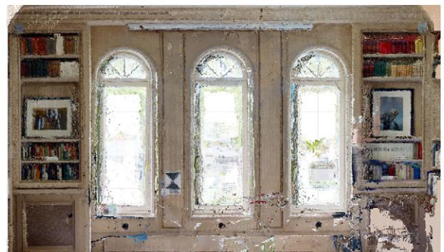
Fig. 2.2.25: .E57 pointcloud with higher point density
