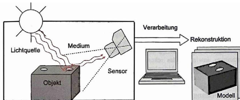
Fig. 2.4.3: From object to result <sup>4</sup>
