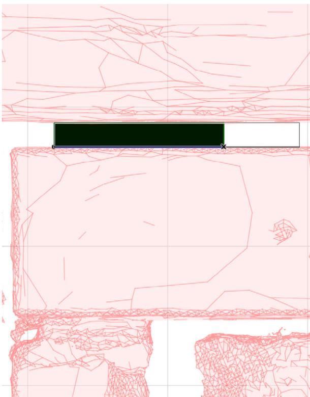
Fig. 3.6.39: Screenshot Archicad, drawing walls based on scan
