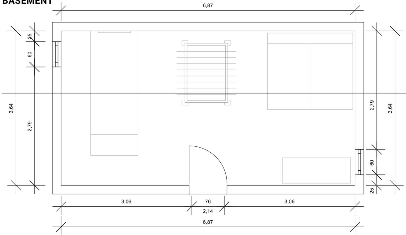
Fig. 2.4.29: CAD Plan view of the Basement
