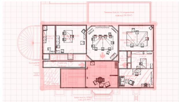
Fig. 2.6.65: Screenshot Archicad, overlaying scans and floor plans
