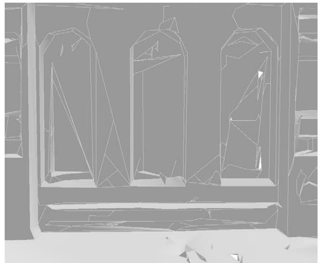
Fig. 2.2.33: Missing window sills of the .3dm mesh
