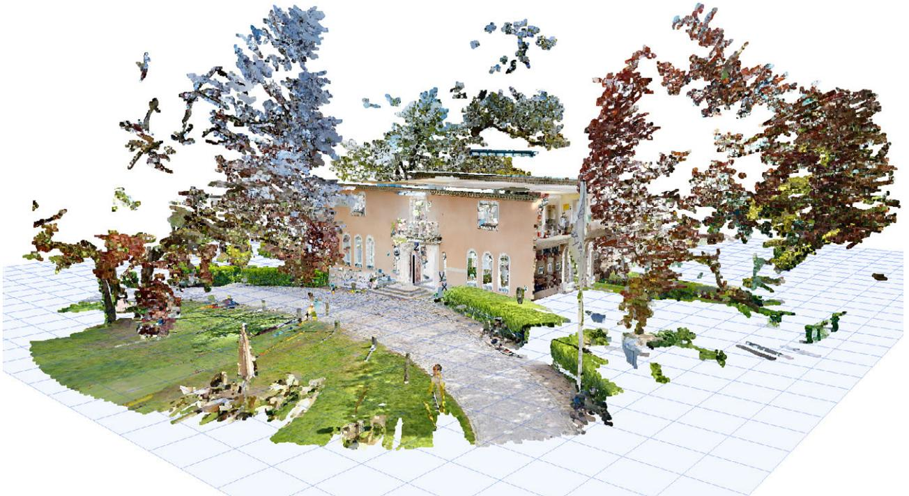
Fig. 2.2.36: 3D-View of .XYZ pointcloud in Archicad
