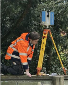
Fig. 1.2.3: IMAGER 5010 on tripod
