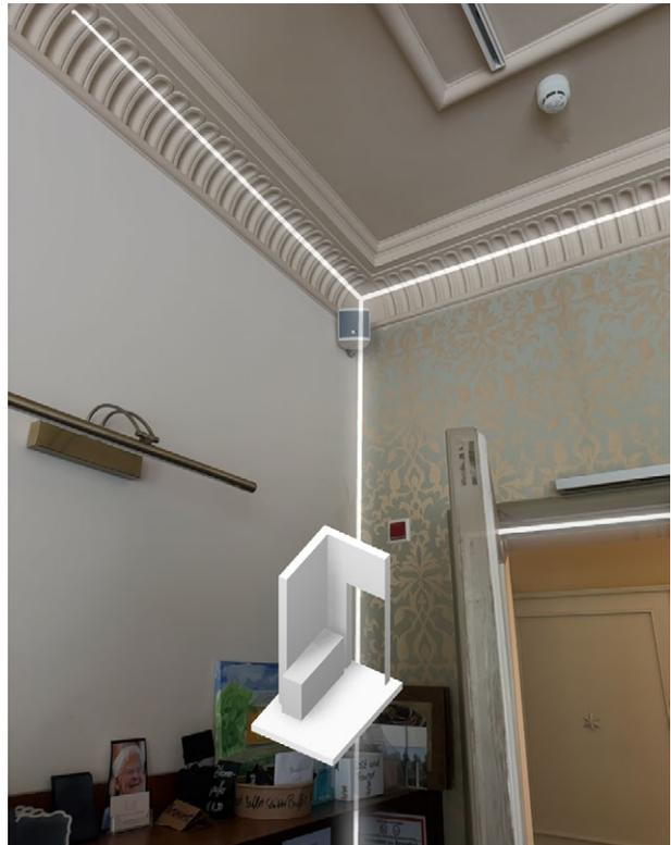
Fig. 2.6.49: Screenshot PolyCam, scanning of stucco moldings
