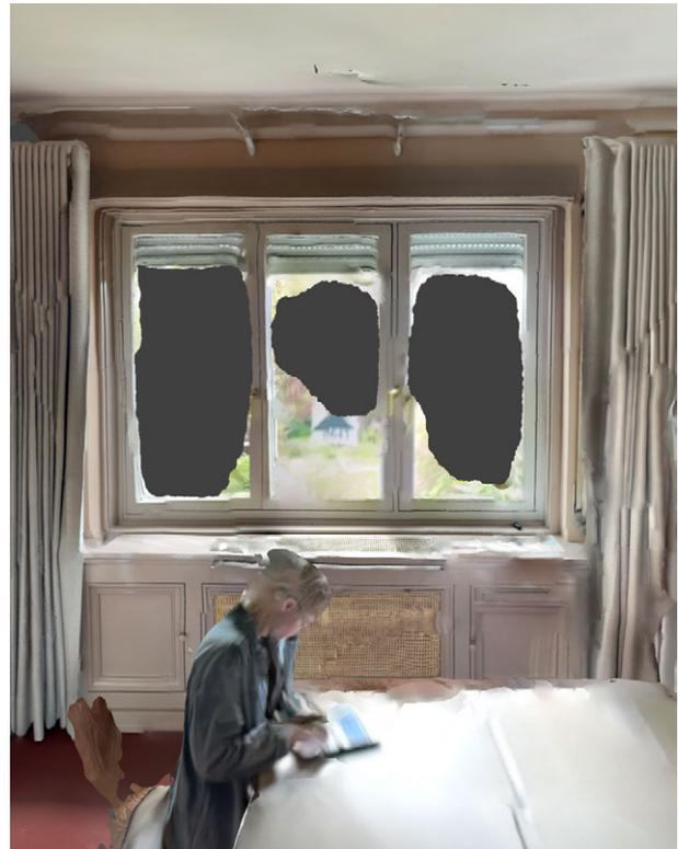
Fig. 2.6.20: Screenshot Scaniverse, holes in scan of window
