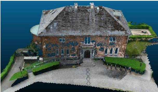
Fig. 1.2.7: Segmented point cloud from photogrammetric image data
