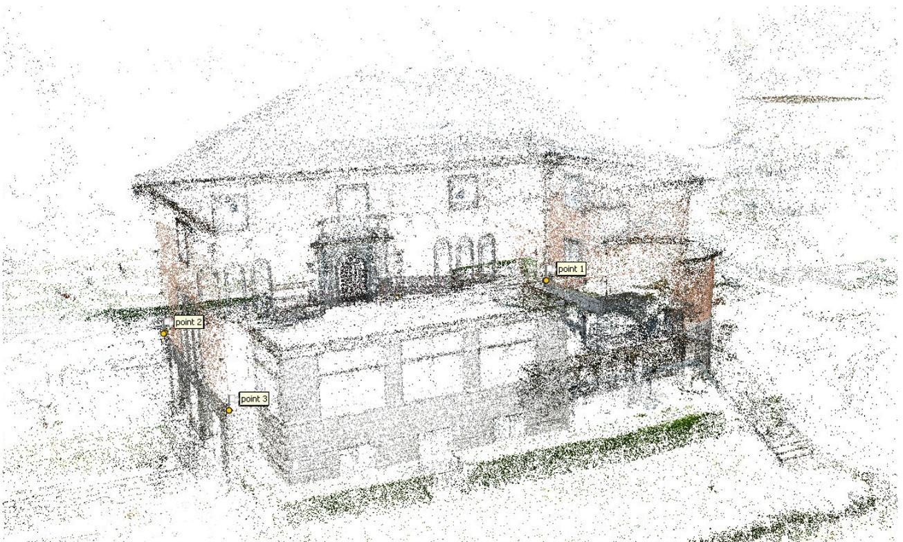
Fig. 1.1.5: Photogrammetry: Light point cloud
