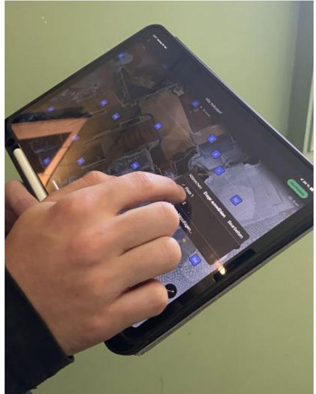
Fig. 2.2.11: Selecting 1F in the Storey Selection Tool the Matterport app
