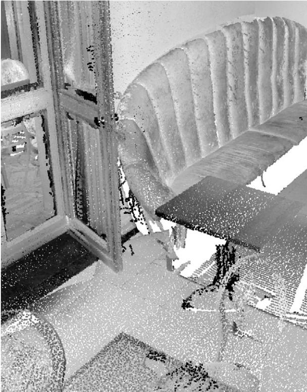
Fig. 2.1.16: Point cloud of the library with a resolution of 3mm
