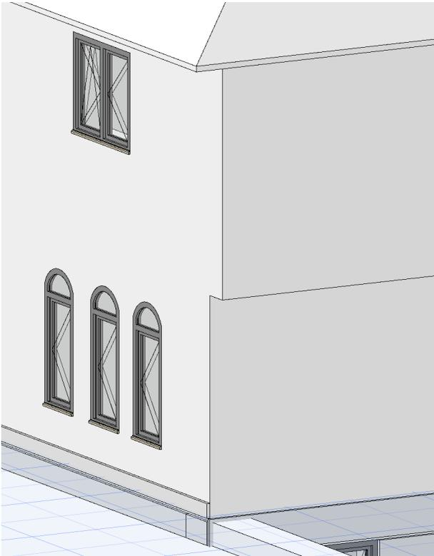
Fig. 2.6.40: Screenshot Archicad, misalignment of the exterior walls
