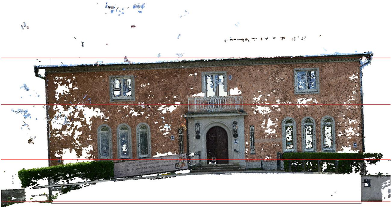
Fig. 2.3.15: Tilt of the North Facade in Point Cloud 1
