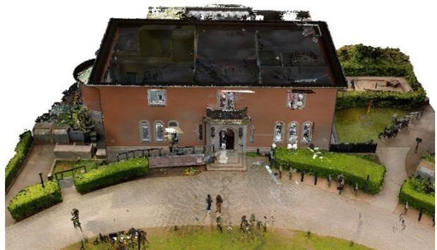
Fig. 1.2.8: Coloured partly segmented point cloud from NavVis VLX 2.0
