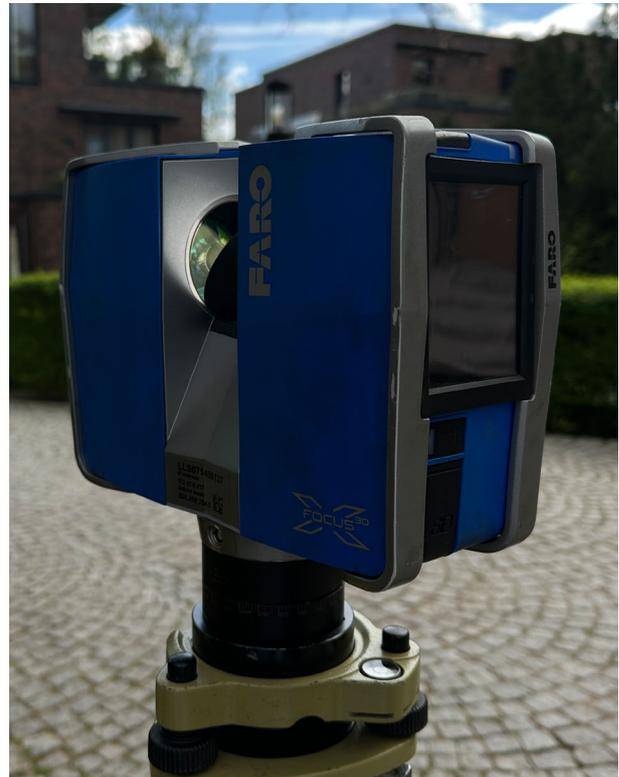
Fig. 2.1.7: FARO 3D laser scanner X30
