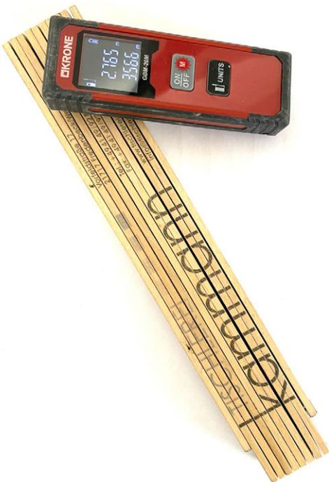
Fig. 2.7.1: Inch rule and laser distance meter
