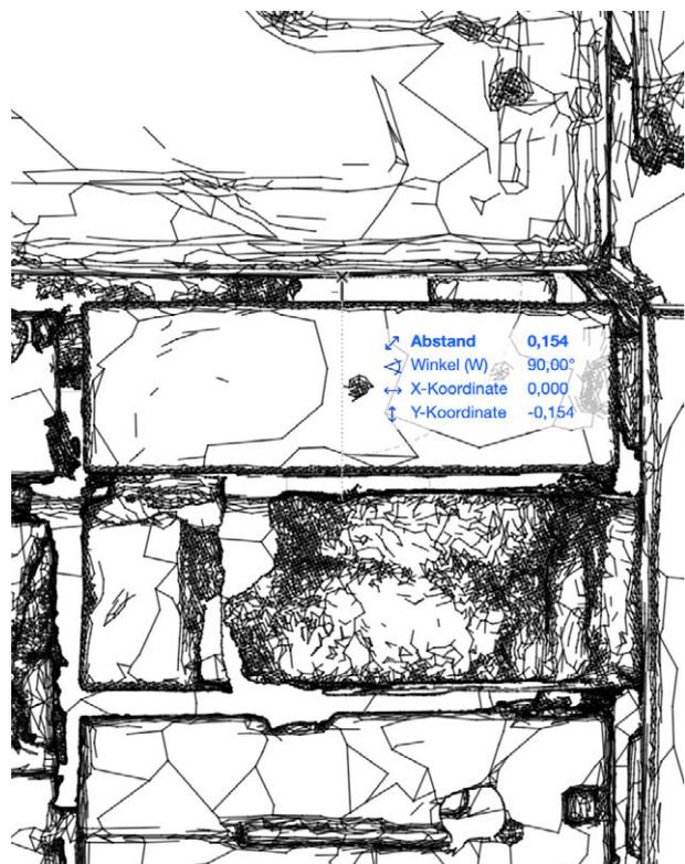
Fig. 2.6.37: Screenshot Archicad, measuring the wall thickness
