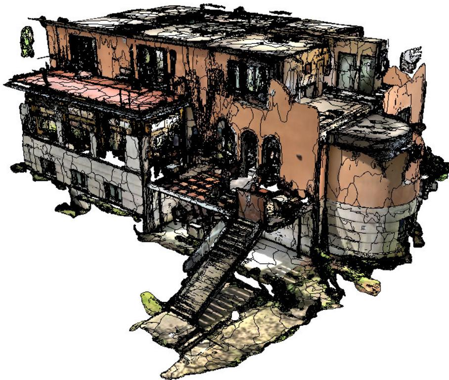
Fig. 2.6.31: Screenshot Archicad, final version of assembled scans
