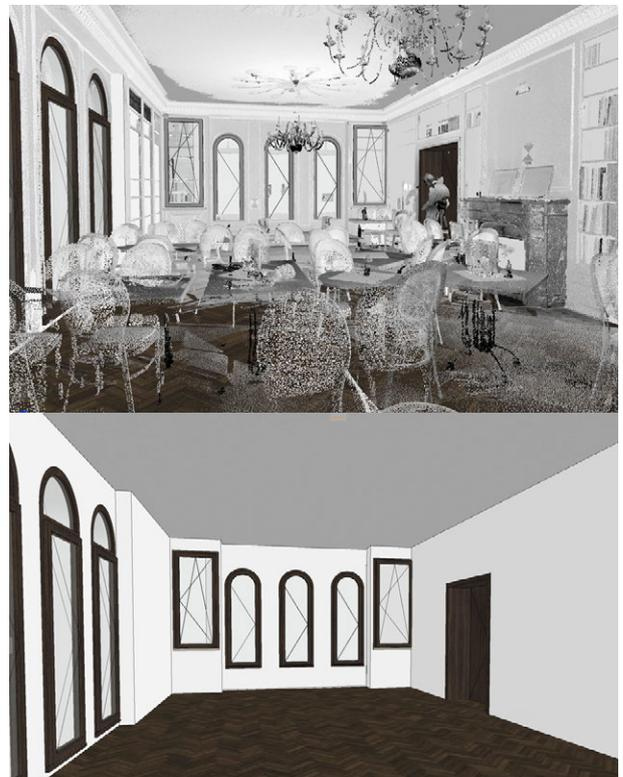
Fig. 2.1.20: Point cloud with the model and the model without point cloud
