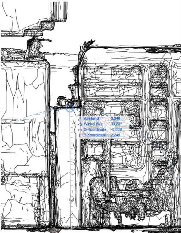
Fig. 2.6.42: Screenshot Archicad, measuring the window height
