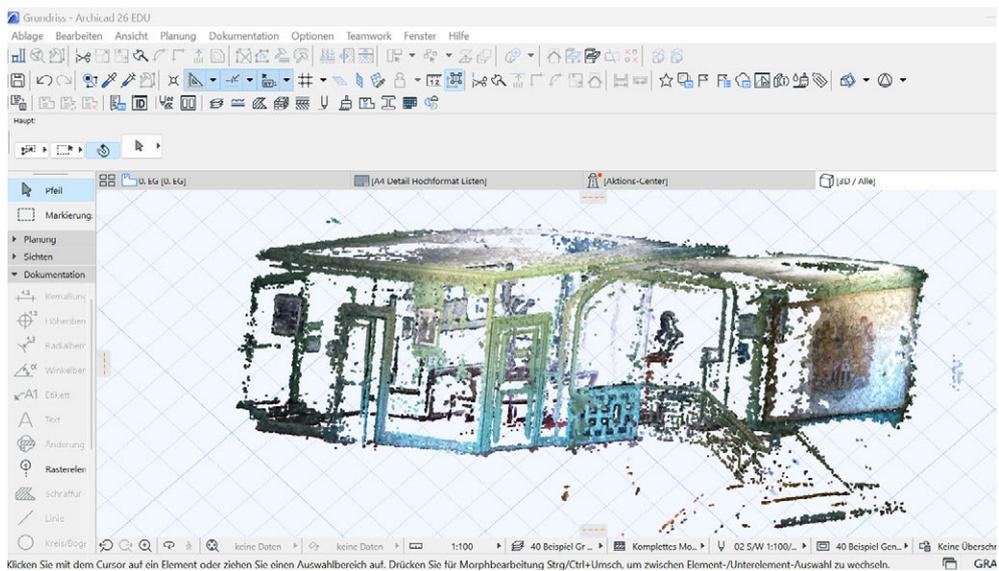
Fig. 2.5.19: Import Model to ArchiCad, 3D Mode
