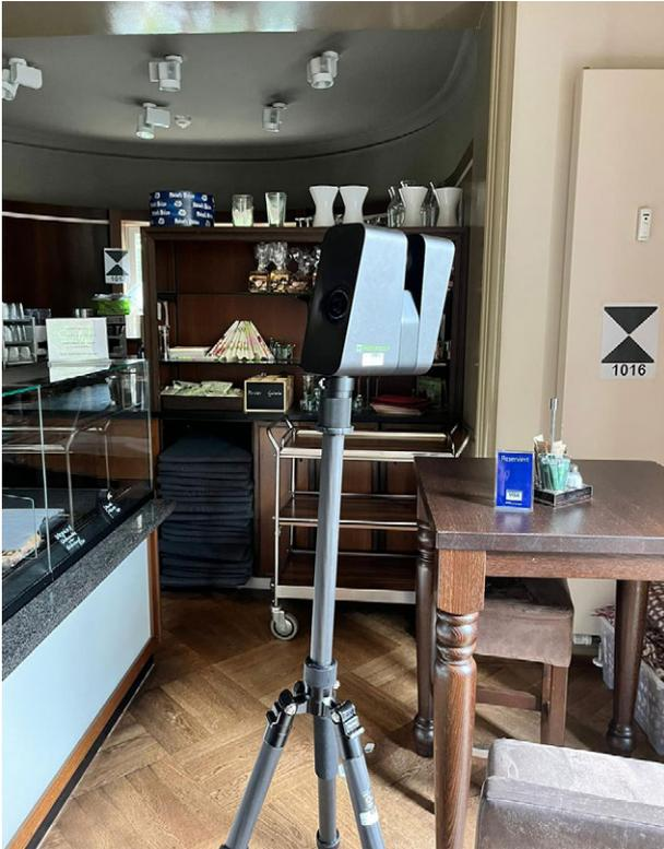
Fig. 2.2.12: Matterport Pro 3 mounted on a tripod
