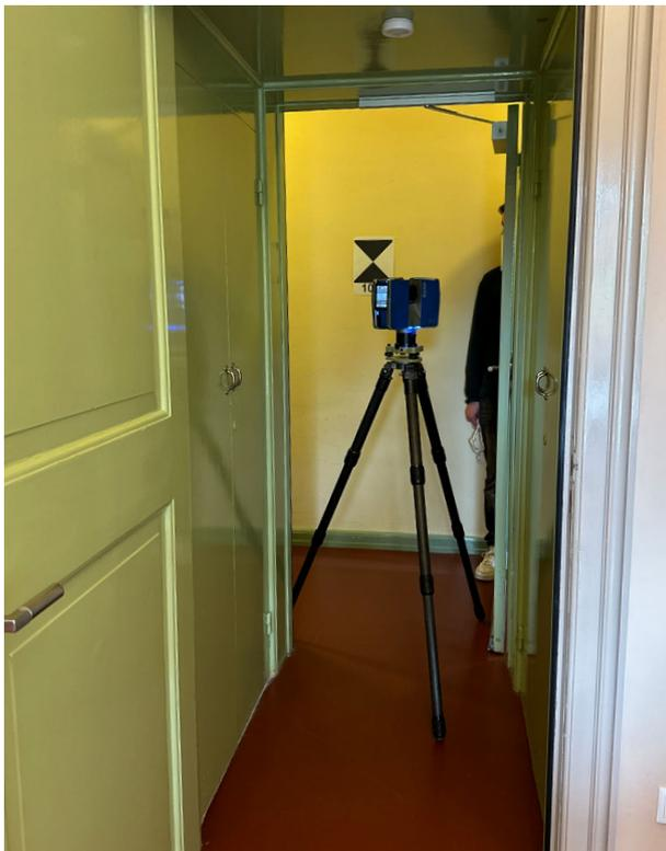
Fig. 2.1.11: The 3D laser scanner at the doorway of a narrow passage.
