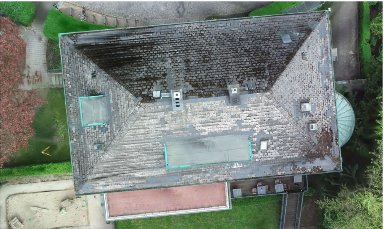
Fig. 1.1.10: Full 3D model using NERF technology - top view
