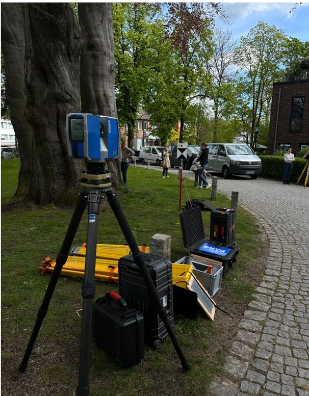
Fig. 2.1.1: Laserscanner Faro Fokus X30
