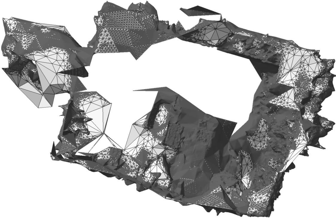
Fig. 2.4.16: 3D Meshes with 3DF Zephyr of the Office Room
