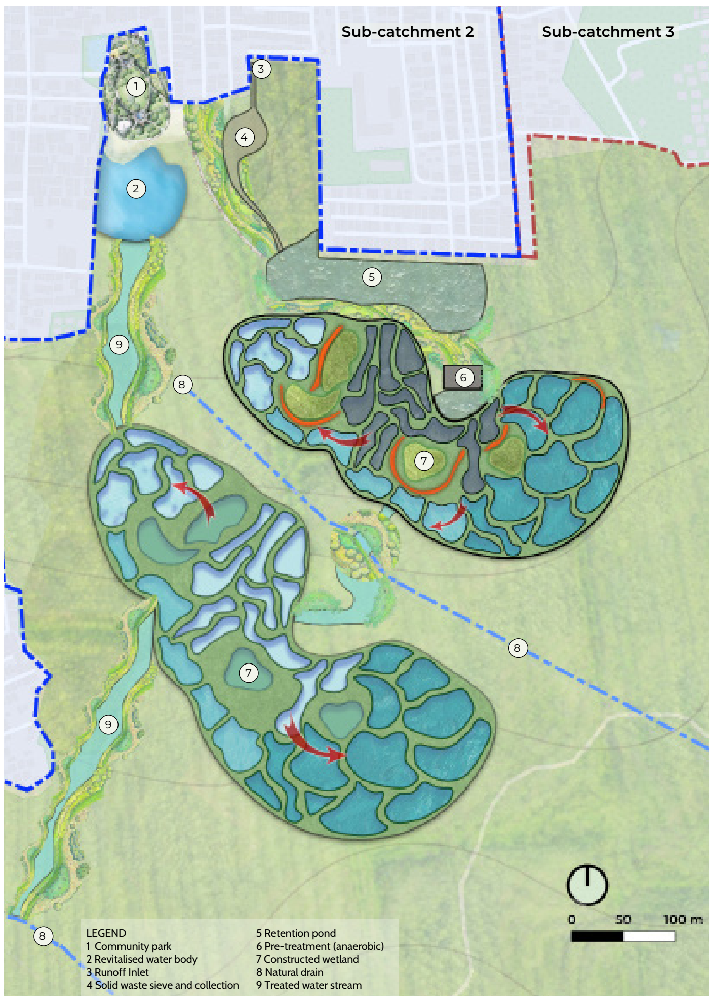
Figure 6-29: Concept design: site plan of the proposed intervention (community area and the constructed wetland)
