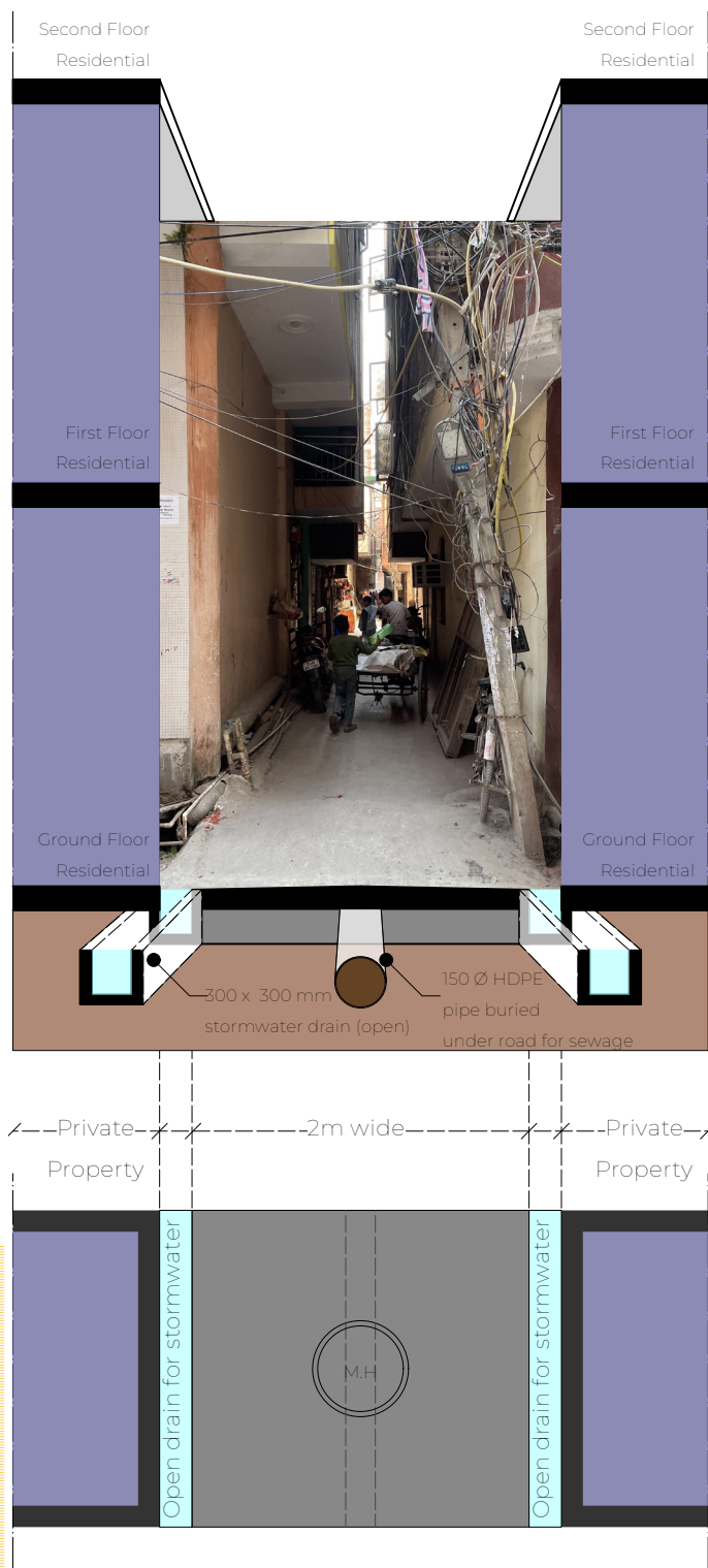
Figure 6-17: Sangam Vihar - Cross sectional view of tertiary street
